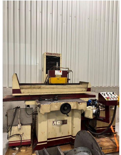
Surface grinder Acer, mod. AGS1224 AHD, table 12" x 24", 5 hp
