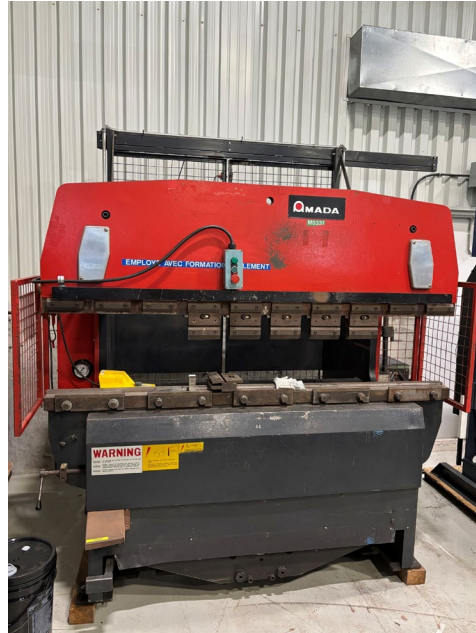
Presse plieuse Amada Promecam RG50, 1995, 6', cap. 50 tonnes, 82.1", 223 volts
